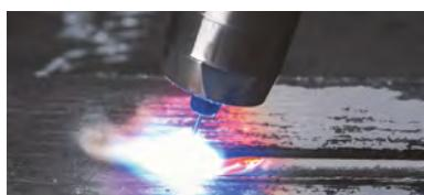
An electric arc forms between a consumable wire electrode and the workpiece (*metal*) which heats the workpiece metal causing them to fuse. The arc and weld pool are shielded by an inert or active gas. Metal is transferred in the form of drops through the arc towards the workpiece. This welding process is used for welding of carbon steel, stainless steel, aluminium, copper...
