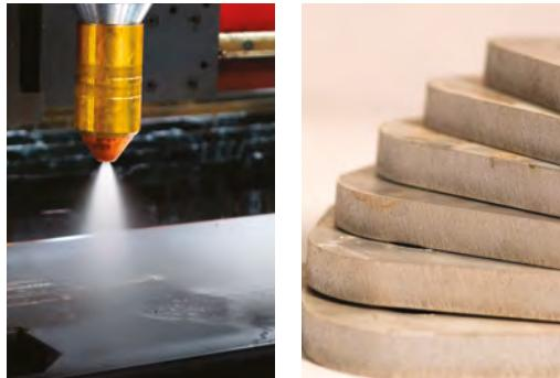
The FineLine® Advanced Process Controller provides the most advanced technologies with water injection. Water injection increases speed when cutting stainless and aluminum, significantly reducing gas cost and improving cut edge quality, with less dross formation.
