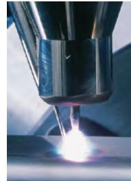
Based on principle of TIG process, an additional filler metal is fed through the nozzle directly into the arc with an angle of 20° to the electrode. This concept guarantees a high deposition rate and an efficient metal transfer. This welding process is used for welding of carbon steel, stainless steel, titanium, inconel, electro-galvanized coated steel (*brazing*)...
