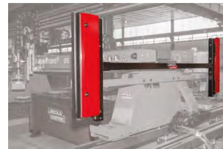
Operator protection customizable depending the implantation of the machine inside the customer workshop to ensure safety and be compliant with machine regulation.
