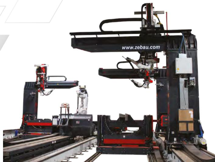
The **Steel Beam Assembler (SBA)** is a fully automated structural steel beam assembly and welding production line. The machine can fit and weld large amounts of steel accurately and efficiently.
