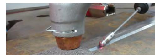
Similar to MIG/MAG welding, SAW involves the formation of an arc between a continuously fed wire electrode. Covering flux is used to generate protective gas and slag protecting the weld metal. The flux can also help donate alloying elements. It is dedicated mainly for flat and fillet welding. This process is generally used for the welding of materials as carbon steel and stainless steel.
